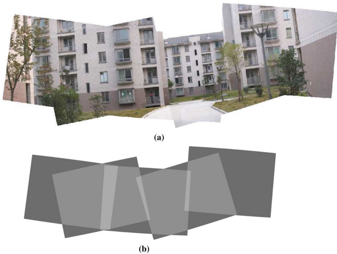
Fig. 14 The stitching result of images in Fig. 12. a The stitching result. b The mask image showing the position and shape of each stitched image in Fig. 14a
